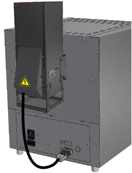
Catalytic converter with fan for removal of organic components from the exhaust air. Organic components are catalytically oxidized at about 600 °C, broken into carbon dioxide and water vapour. Irritating odors are thus largely eliminated. The B400 - P480 controllers can be used to switch the catalytic converter automatically (not for models L(T) 15.., L 1/12, LE 1/11, LE 2/11).*
